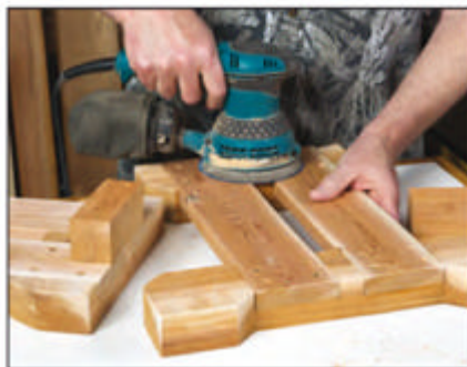
Before attaching the mounting cleats, sand the cleat location flush, if needed, to ensure a secure attachment.
