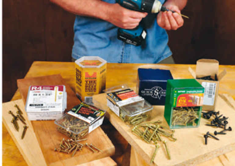
Originally developed for the building and wood products industries, production screws, as well as construction and deck screws, are made from carbon steel heat treated to provide a good balance of hardness and toughness.
