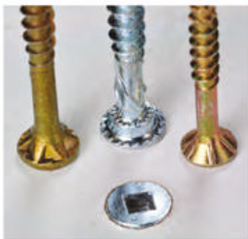
The underside of the heads of (left to right) the SPAX MULTI Head, Quickscrows' Funnel Head and GRK's R4 has nibs or serrations that slice into the surface to create their own recess.
