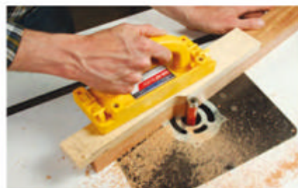
The cloudlift leg profiles are best made against a template secured with double-sided tape. Use a piloted flush-trim bit to follow the template.
