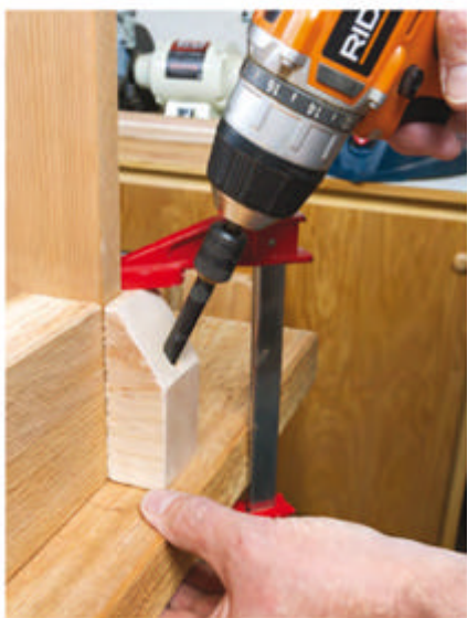
For the outer edges of the last boards, countersink diagonal pilot holes through the bench and table end pieces, and secure with screws.
