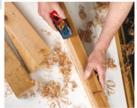
The author chamfers the corners of his cedar components. It not only helps to prevent splinters, but it looks great, too.
