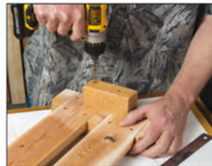
Center the mounting cleats on the inside tops of the table and bench end assemblies, and secure with weatherproof glue and exterior screws.
