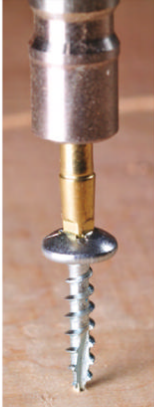
The sharp Type 17 auger point found on most production screws enables the screw to quickly penetrate most woods without the need for a pre-drilled pilot hole.
