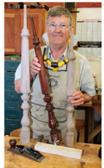
When he turned six replacement balusters with tapered octagonal sections, the author found the turning easy. The difficult part was tapering the octagon, which he did at the bench with a #97 plane.
