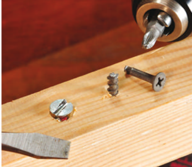
Old-fashioned tapered steel wood screws are made from relatively weak steel, so their slot recesses tend to deform and cam out. The shanks of drywall screws often snap when driven with ambitious force.
