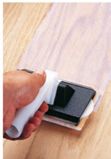
A paint pad provides a larger surface than a brush for applying water-based finish — it's easier to apply a smooth, thin layer.
