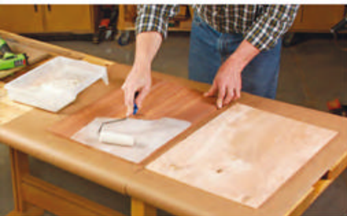
Roll wood glue onto the side panel veneer and its substrate, then assemble the lamination and tack near one edge to keep the panels aligned.
