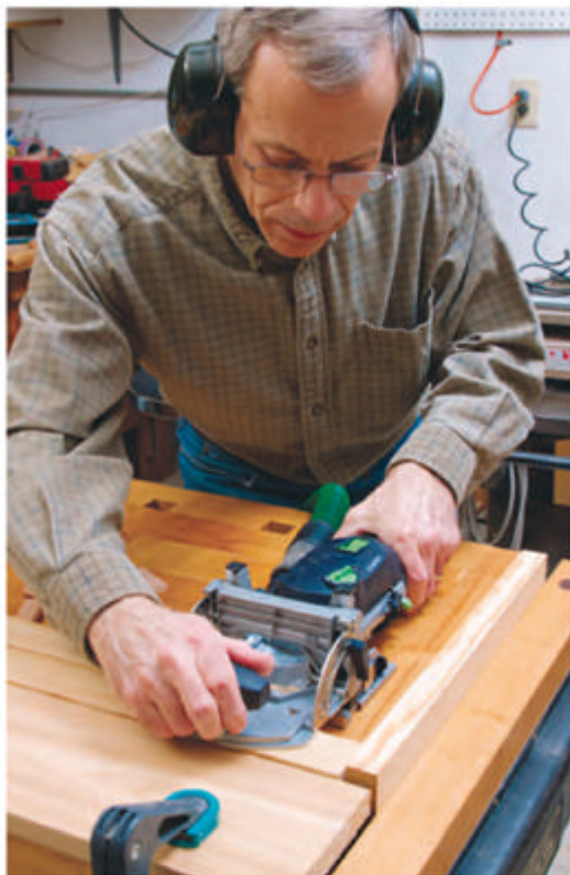
A Festool Domino is a quick way to make strong mortise-and-tenon joints for the shutter frames. Dowels, plate-joining biscuits and pocket-hole screws are good alternative joining methods.
