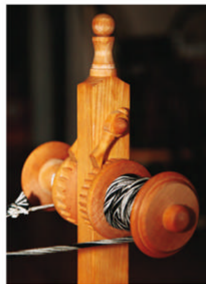
These ratchet pawls are on a Swedish band loom. The tall column to which the pawls are attached is square with the top section turned: it is flat/round.
