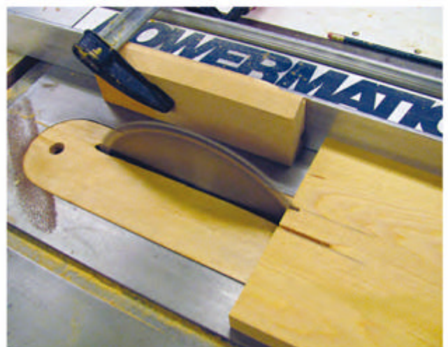
The notched joinery on the legs and upper stretcher can be formed using a table saw (as shown above), or cut by hand. The lower stretcher is held in place with dowels.
