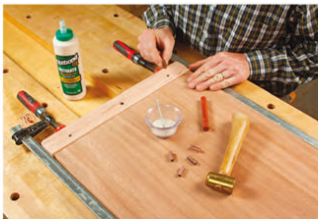
Square pins driven into the breadboard ends and through the panel tenons fasten the parts together. The outer pegs fit into slotted tenon holes.
