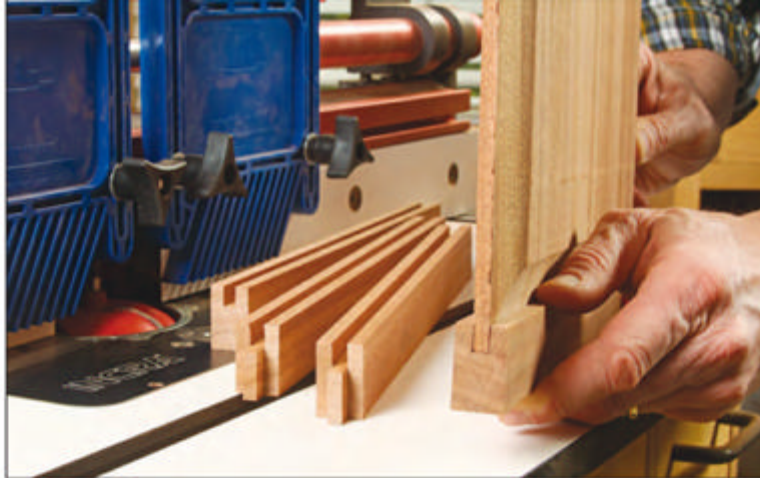
A large raised-panel cutter with a cove shape reduced the door's 1/2"-thick panel to fit the frame grooves while also adding a decorative profile around its face. Take several rounds of deepening passes for safety and to help minimize burn marks.
