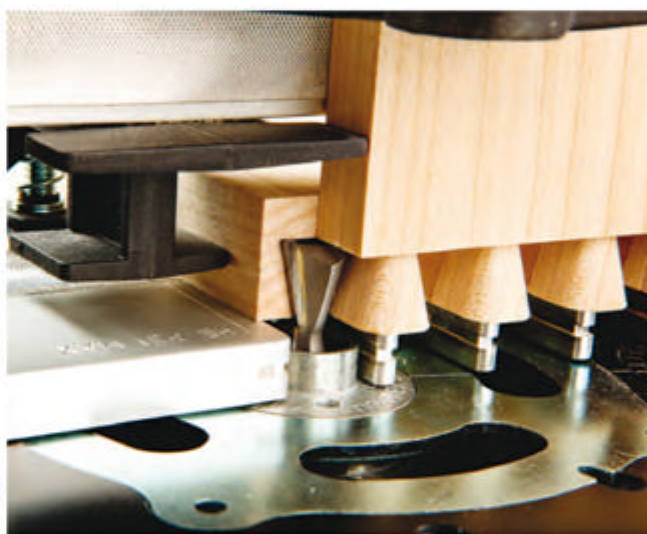
Stepped side stops position pin and tail boards accurately — very helpful for half-blind dovetails where both joint parts are milled simultaneously.
