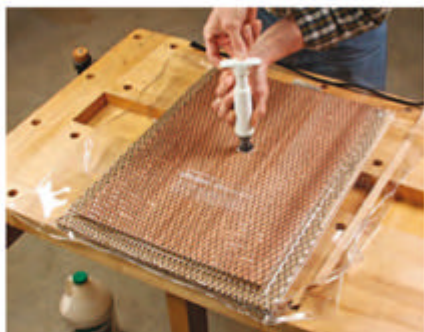
A heavy-duty vacuum bag, one-way valve and hand pump made easy work of pressing the side panel veneers flat against their substrates.
