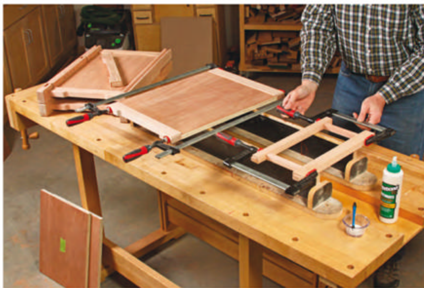
The back panel and rails form a third major subassembly, while the top and middle front rails and full slats make a fourth subassembly. Gluing these parts together now reduces the total number of wet glue joints in the final big carcass glue-up — and that makes the whole assembly process easier.
