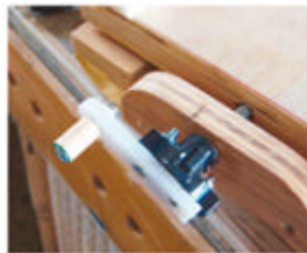
Raymond LaRochelle upgraded the adjustment system of his Framing Jig by adding a crank.
