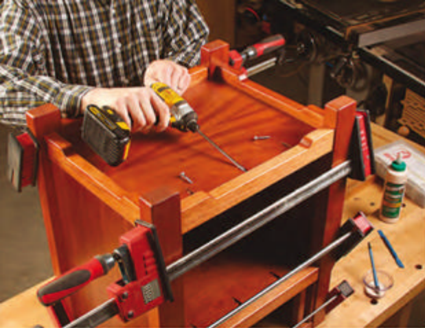
Pocket screws driven from the bottom panel and fixed shelf into the front bottom and center rails strengthen these joints and ensure that the visible seams are tight from above.
