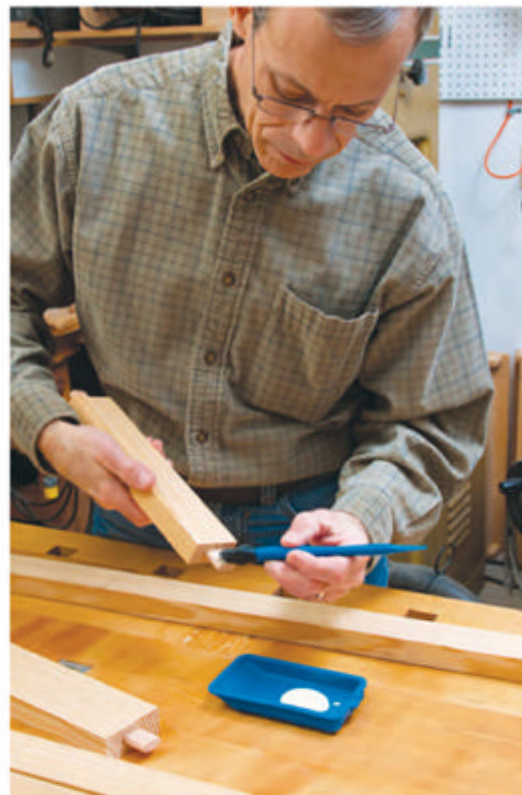
When assembling the frames, spread glue evenly inside the mortises and on the tenons. A silicone brush works well here and can be easily cleaned because glue won't adhere to it.
