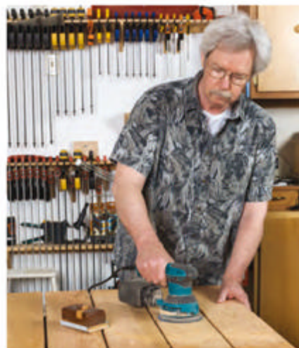
To avoid getting splinters during use and to help make the table and bench tops easier to clean, sand the rough surface smooth.
