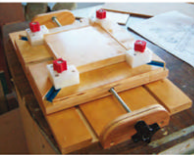
Raymond LaRochelle upgraded the adjustment system of his Framing Jig by adding a crank.
