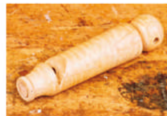
The fiddle plug for the mouth-piece of whistles and recorder flutes (seen above) has to have an exactly sized flat spot so the right volume of air hits the sharp edge of the bore.
