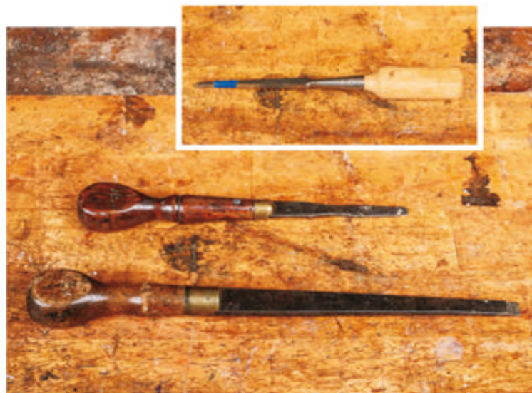
The handles on these antique screwdrivers were made with flat spots, which tell the user the alignment of the top and provide more purchase to torque screws home. After first turning a handle with flat spots, it's easy to make it into an oval handle (see inset) by rolling the flats against a belt or disc sander.
