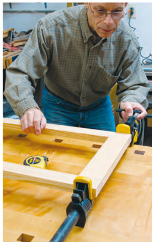
Clamp the frames with even pressure applied on the center of the joints. Check for square by measuring diagonally across the frame from corner to corner with a tape measure.
