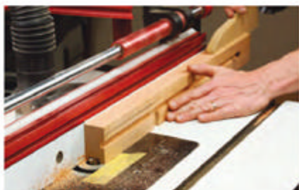
Mill the front legs' rail mortises at the router table with a 1/2" straight bit. Mark the bit location on the table to guide these "drop" style cuts.
