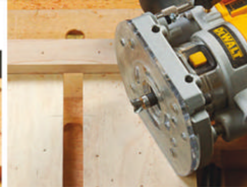
A clamp-on routing jig, with a slot sized to match the fixed shelf and bottom panel plywood thickness, ensures accurately made dados in the legs. The author used a piloted hinge-mortising bit (see inset) to mill these 1/4"-deep, 1"-long cuts. A back stop on the jig limited the cutting length.
