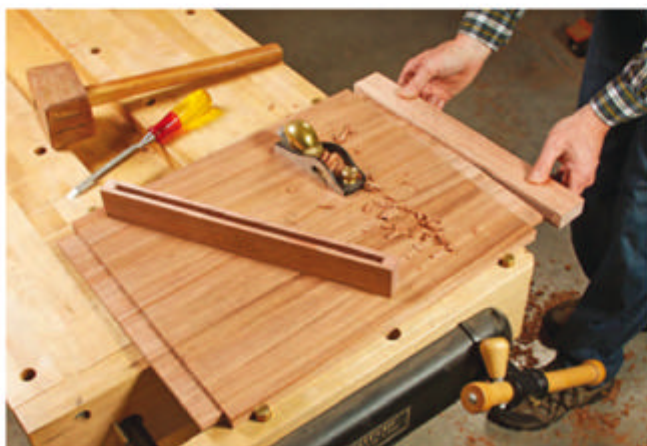
Continuous tenons on the ends of the top panel fit into matching mortises in the breadboard ends. Aim for a snug friction fit of these joints.
