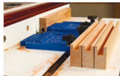
The side panels require two different groove depths in the side rail blanks (shown): 1/2" deep for the bottom rails; 3/4" deep for the top rails.
