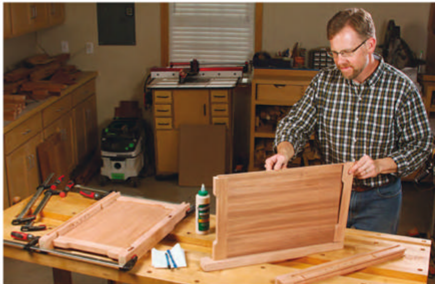
Form two side assemblies by gluing the legs, side rails and panels together. Glue the side panels into their grooves — their veneer/plywood construction makes wood movement a nonissue here.
