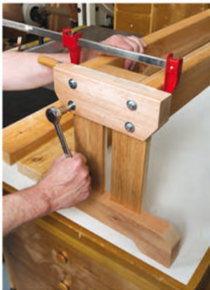
Drill a pair of 1/4" pilot holes for each stretcher through the bench and table ends, then drive home 4 1/2"-long lag bolts for a solid frame.
