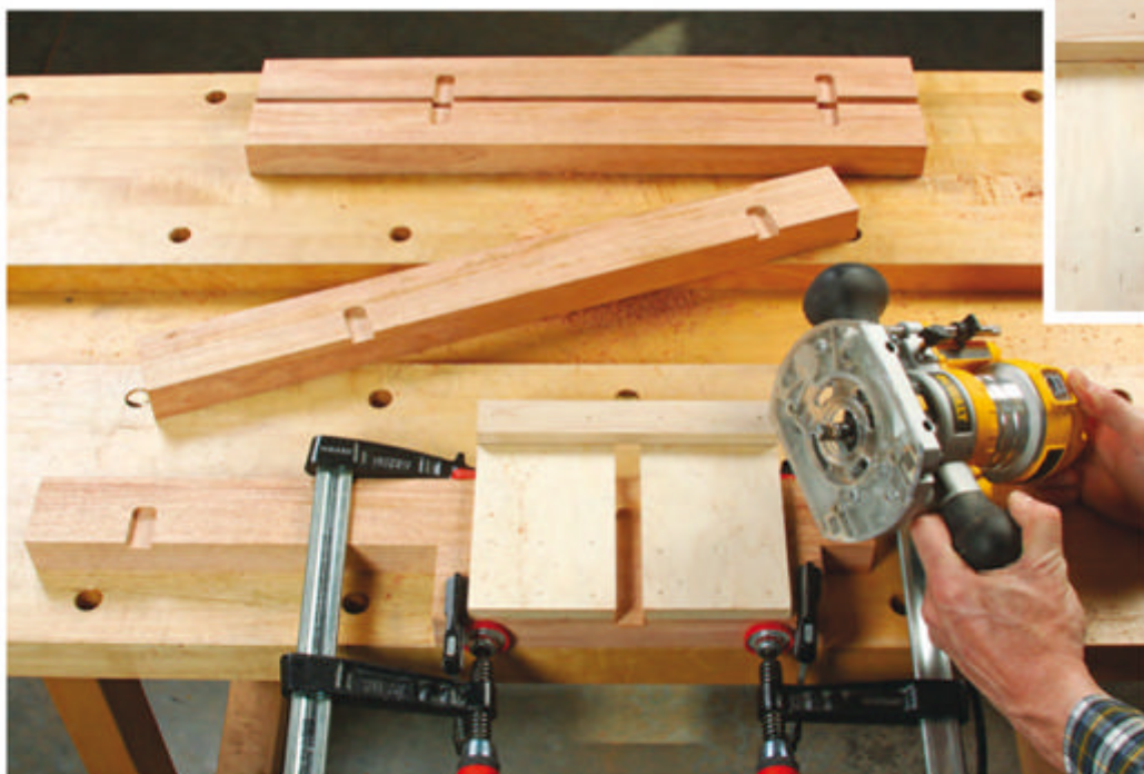
A clamp-on routing jig, with a slot sized to match the fixed shelf and bottom panel plywood thickness, ensures accurately made dados in the legs. The author used a piloted hinge-mortising bit (see inset) to mill these 1/4"-deep, 1"-long cuts. A back stop on the jig limited the cutting length.
