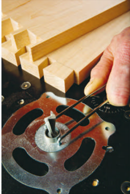
Numeric indexing on Leigh's "e10" eBush makes adjusting the fit of a joint's mating parts as easy as twisting the elliptical bushing left or right and re-routing one piece.
