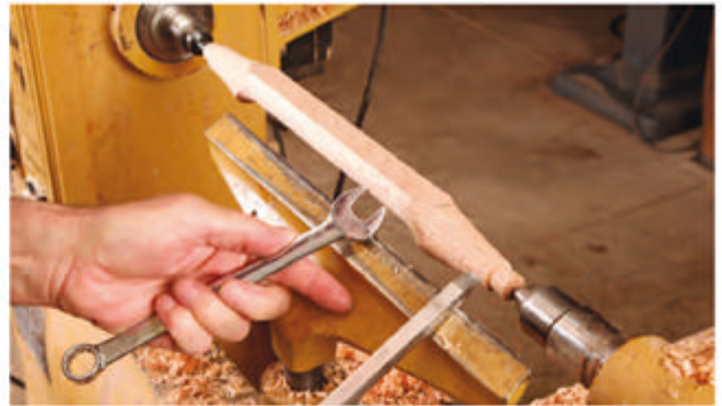
The author turned the stretcher on this three-legged stool in two axes, with an intentional flat spot meant to serve as a footrest.
