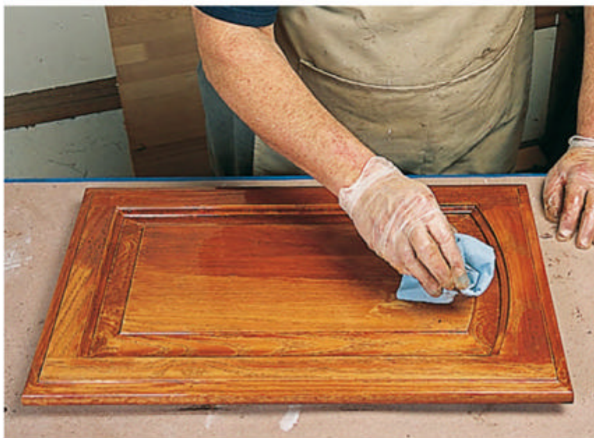
A paint pad provides a larger surface than a brush for applying water-based finish — it's easier to apply a smooth, thin layer.
