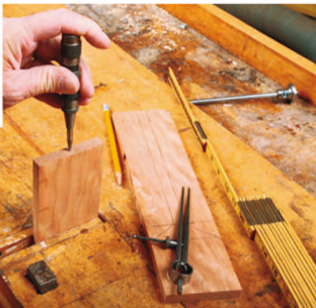
For relatively flat boards that are going to be turned into things like salad forks, dividers and a marking gauge (seen in the tool well in the photo above) give speed and accuracy to finding the center and the layout.
