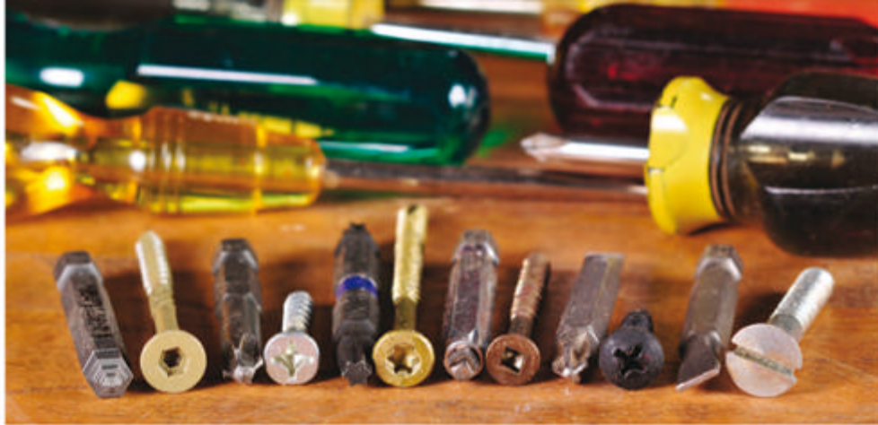
Wood screw drive and driver styles include (left to right): Outlaw, Posisquare (combo), TORX (star), Robertson (square), Phillips and traditional slotted (which are most prone to coming out: the driver slips out of the screw head, distorting the slot).
