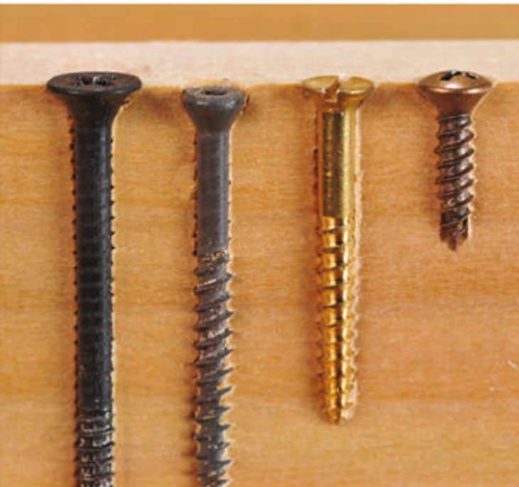
Screws with heads that sink flush (or near flush) with the work surface are, left to right: bugle head, trim head, flat head and oval head.
